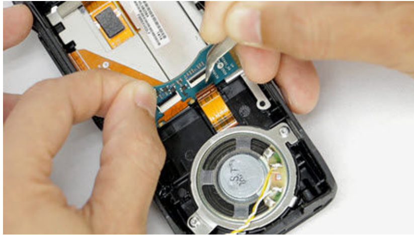
11 Disconnect the GCAI flex from the interface board.
